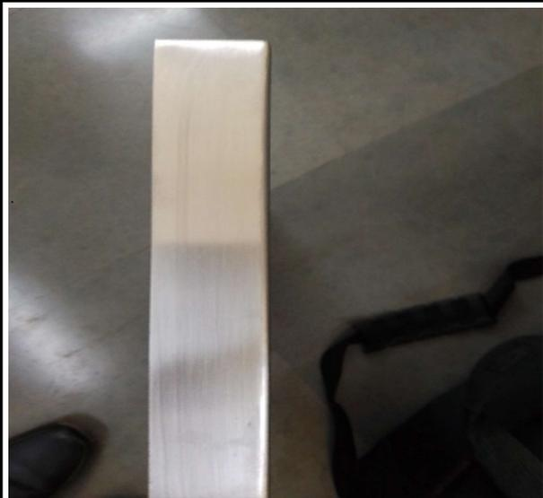
A photograph of the same autoclave tool after cleaning. The surface is now bright and reflective, with all the corrosion removed.                                                                                                      |
