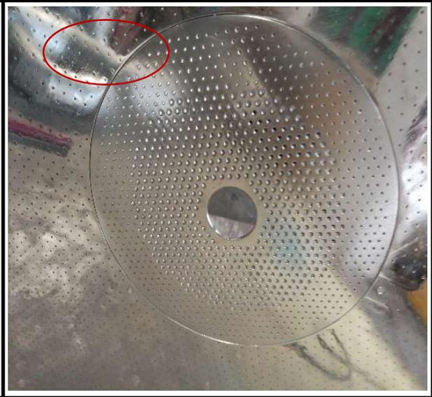
A photograph of the same circular perforated metal filter plate after cleaning. The surface is clean, shiny, and free of the brownish deposit. A red oval highlights the same area as in the 'Before' image, showing the clean metal. |
