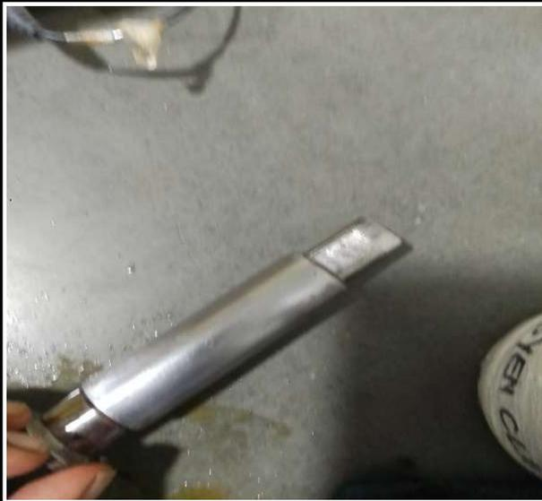
A photograph of the same tablet punch after cleaning. The brown corrosion has been completely removed, and the metal surface is clean and shiny.                                                                                        |
