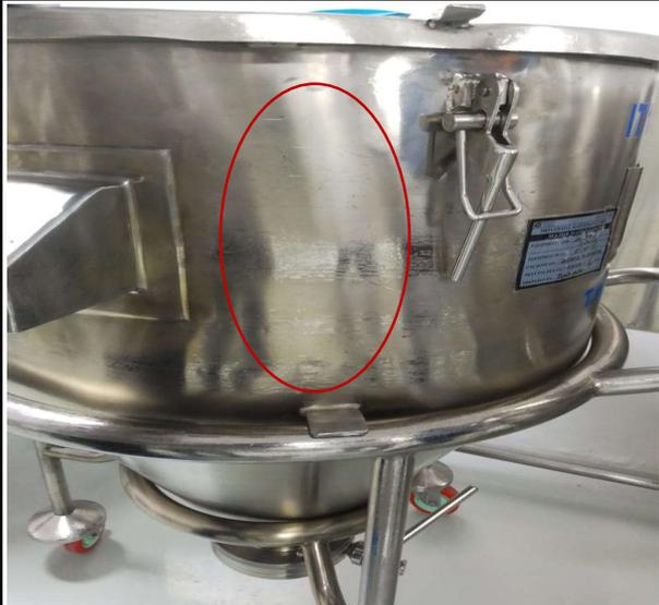
A photograph of a large stainless steel powder handling vessel. The surface is dull and shows signs of corrosion. A red oval highlights a section of the side panel. |                |
